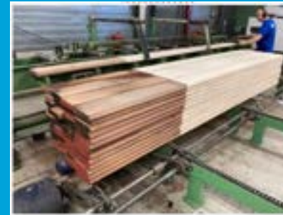
Gevingerlaste combi- damwand Angelim Vemelho-Vuren
