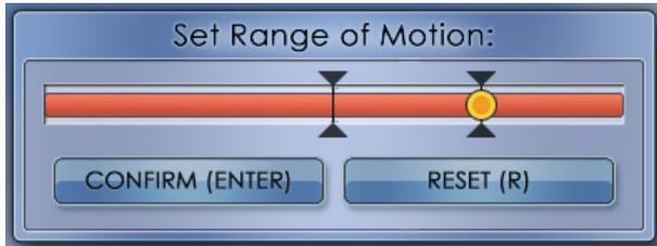
The Min value should be around "0" the max value is the end of the range. If the "min" value is not "0" please reset the electronics (Reset button). Then make the repetition (to set min/max) again, ending in the "min" position.
